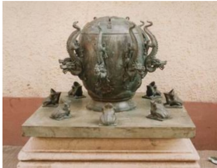
Fig. 1 – Ancient Chinese seismometer. Notice the dragons around the vessel and the toads beneath them.
