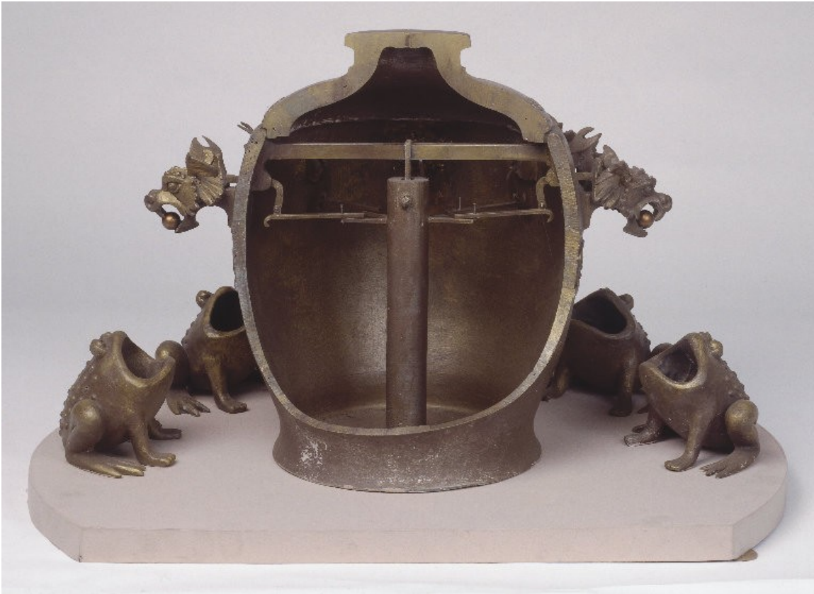
Fig. 2 – A cut-away look at the inside workings of the ancient Chinese seismometer.
